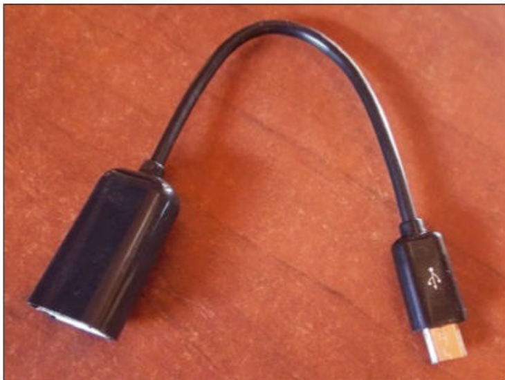
Figure 2: An inexpensive OTG adapter would let you use a Nitrokey with an Android phone.
