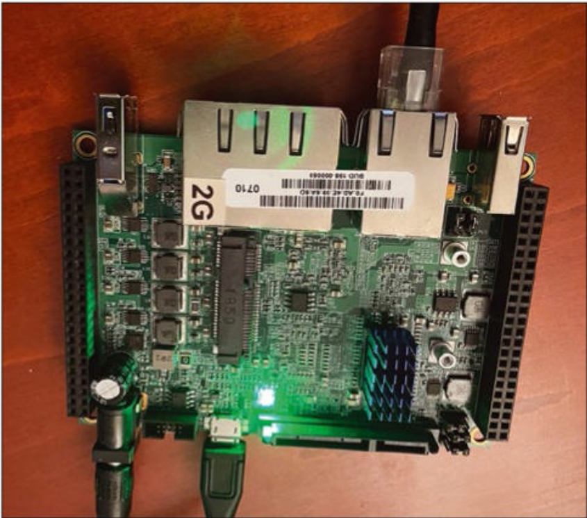
Figure 1: ESPRESSObin v7 SBC shown in the 2GB of RAM and no embedded MultiMediaCard (eMMC) variety.
